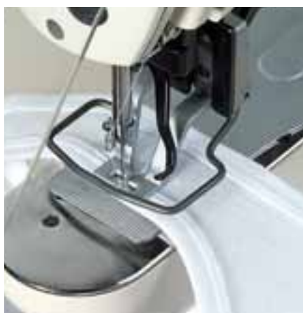
M type (Bartacking shoulder of running shirt)
