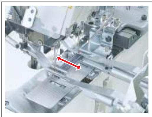
● The widthwise position of the belt-loop can be offset.
