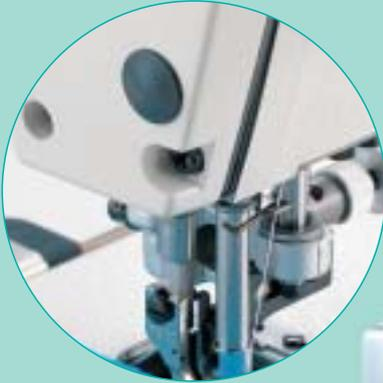
The highly efficient lockstitch machine which assures the consistent quality of finished seams comes with a sharp knife capable of cutting various types of material.
