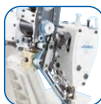
New type belt feed mechanism
