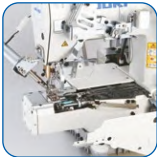
Electromagnetic needle thread / looper thread trimming device
