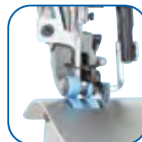
Alternating vertical movement mechanism
